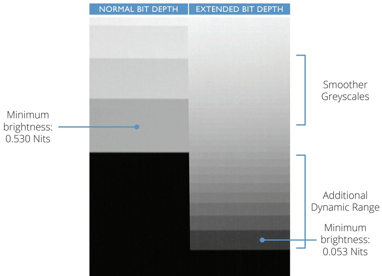
Performance at 0.05% brightness with Dark Magic disabled, illustrating PWM bit depth improvement: Frame grab from camera footage of 2000 Nits panels running at just 1 Nit.
