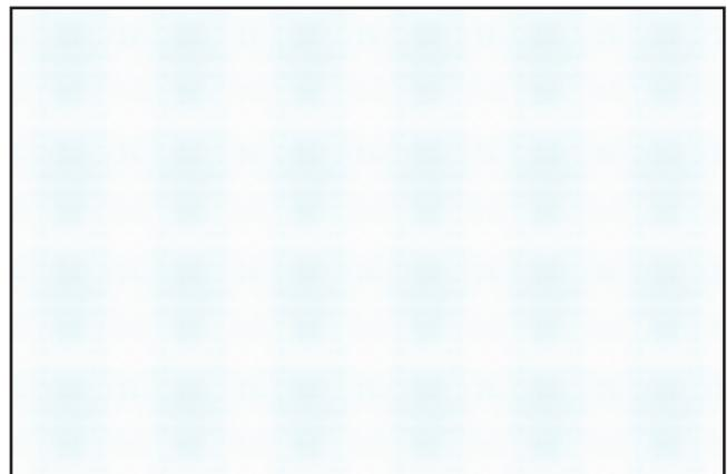
*Uncorrected panels show a regular patterning of cyan colour shift, corresponding to the hotter parts of the screen.*
